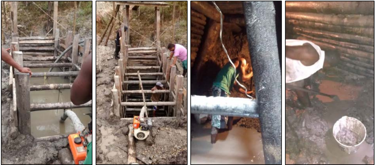
Dewatering underground alluvial workings (Deep Leads) and sampling north of Novita in February 2017
