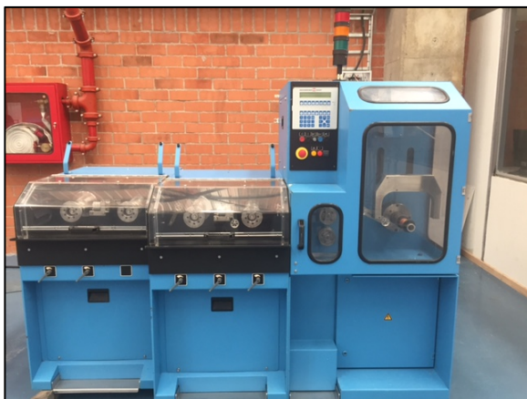
Niehoff automated wire drawing machine/equipment, GPS Metals Lab, Cali Colombia
