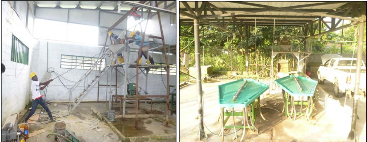
Figure 3: Dismantling gold and platinum processing equipment at Martinez Mine. And re-establishment at Novita Compound, green Gemini Tables now operational,
