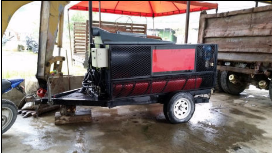
Figure 1: New Mobile Alluvial Processing Plant, rated for 1 tonne per hour
