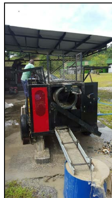
Figures 8 and 9: Testing local alluvial material from Novita Community Lands with mobile plant, July 2016
