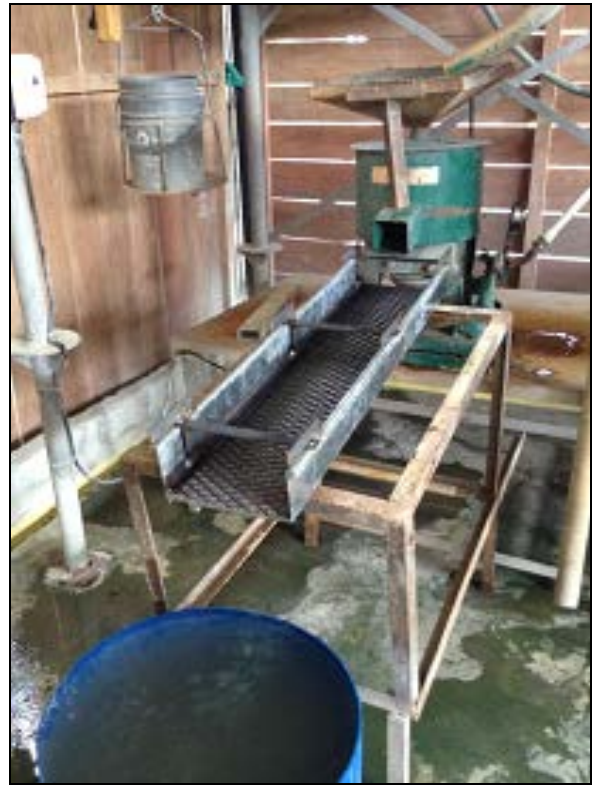
Figures 1 and 2: New inline filters added to Gemini Tables. Small Knelson concentrate serviced, new sluce fabricated. Gold processing plant wet floor now sealed and painted, recycling tanks pumps and filters all operational.
