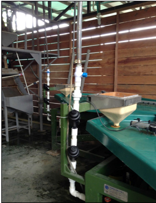
Figures 1 and 2: New inline filters added to Gemini Tables. Small Knelson concentrate serviced, new sluce fabricated. Gold processing plant wet floor now sealed and painted, recycling tanks pumps and filters all operational.
